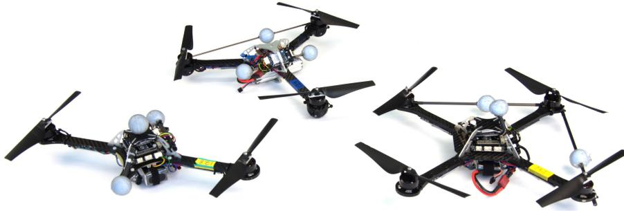
**Fig. 11.** A novel class of flying vehicles, from left to right: bispinner, trispinner, and quadspinner. For each vehicle, all propellers rotate in the same direction, causing the vehicle to rotate in the opposite direction in hover. Extension 2 contains a video showing each of these vehicles flying.
